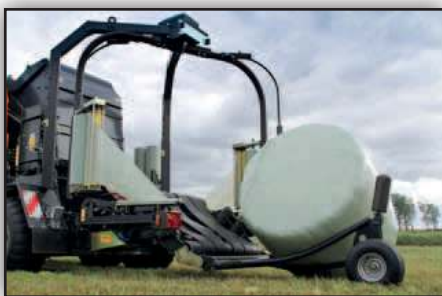
Bale-on-end kit is available as option. During transport the kit is automatically transferred into a safe position inside the wrapping unit.
