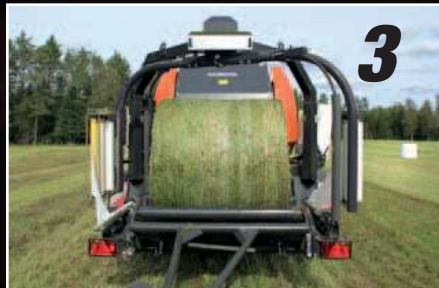
As soon as the bale is transferred away from the baler, the tailgate automatically closes, and baling of the next bale can start.
