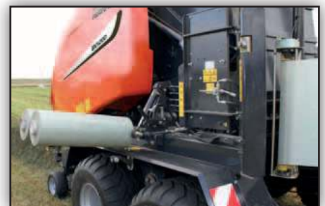
The extra stretch films are lowered hydraulically for easy change.
