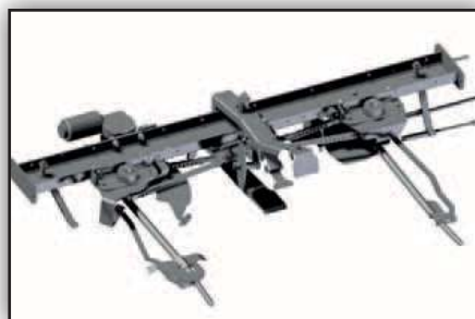
Twin tube fast operating twine binding system.
