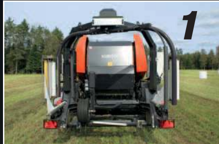
Once the net is applied to the bale the wrapping table is transferred to the tailgate of the baler.
