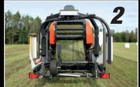
The bale is dropped directly onto the wrapping table.
