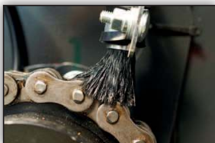
Automatic chain lubrication is standard with lubrication activated continuously at a pre-determined level for each individual chain.
