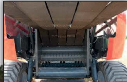
A combination of 5 belts and front rollers provides dense bales with a soft core and a easy bale start.
