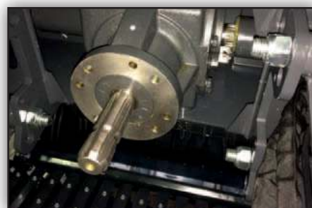
The split drive gearbox ensures that power is distributed evenly, reducing wear and power requirement.
