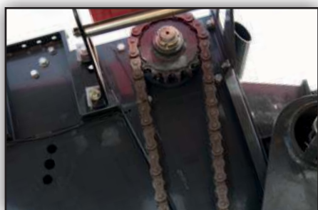
Main bale chamber drive is by heavy duty 1 1/4" pitch chain for longer lifetime and reduced maintenance.
