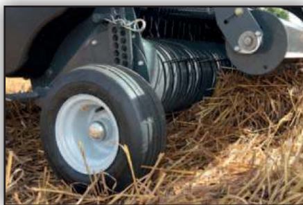
Guide wheels with generous flotation tyres and simple height adjustment.
