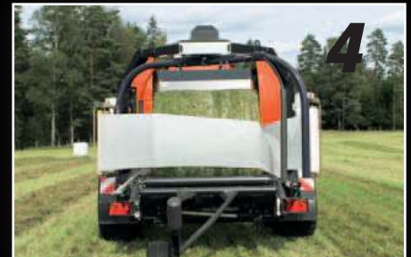
The wrapping table moves very fast to the pre-stretchers and wrapping starts instantly.
