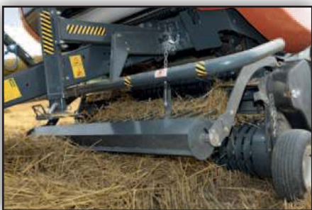
Large diameter roller crop facilitates higher intake speeds.
